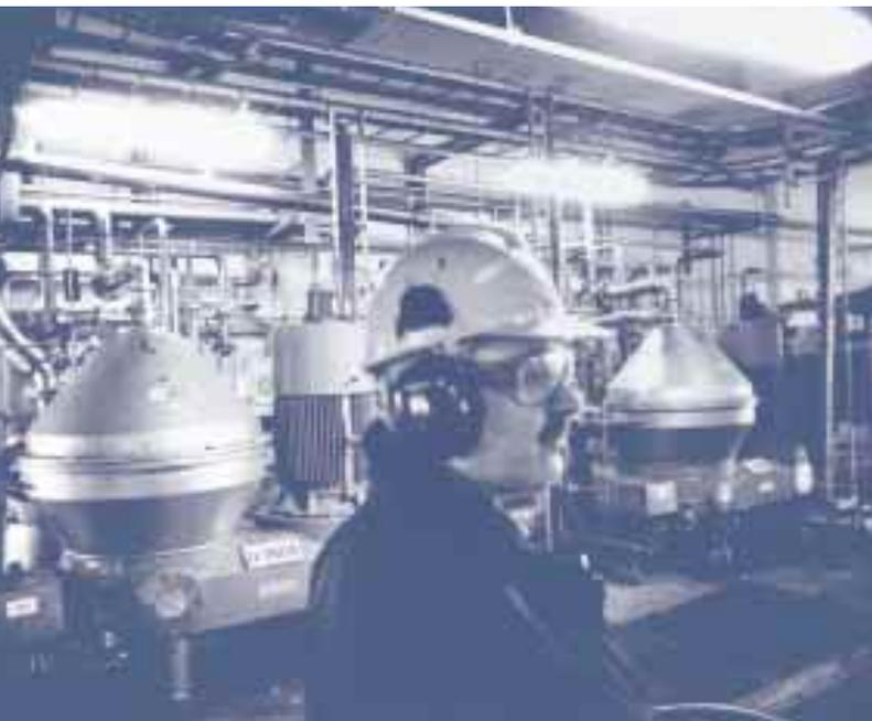
*Kjell Hystestad operates the recovery plant, in which sludge separators are key components. Copper oxide in the sludge is separated from the spent vanillin liquor and recycled. Vanillin liquor is an important raw material for Borregaard's lignin business.*
