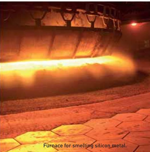
Furnace for smelting silicon metal.
